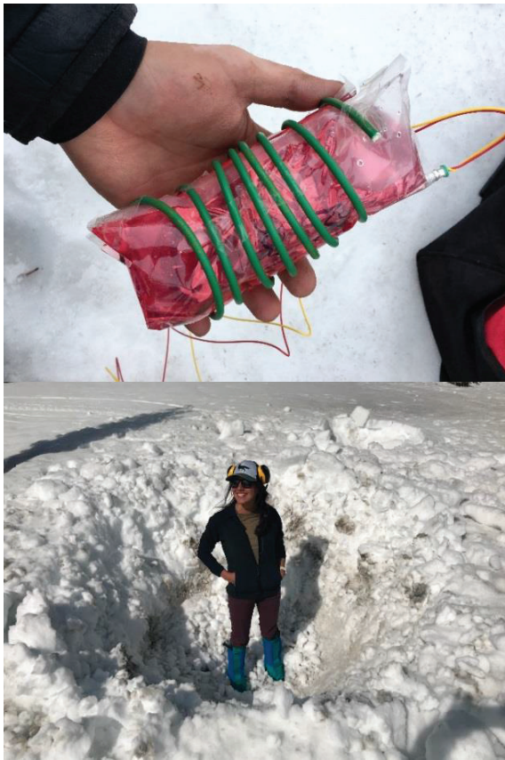
Figure 3. Top, GEM charge contained in a mylar bag and wrapped with detonation cord and #8 denotator. Bottom, heavy wet snow blast crater formed by GEM detonation exhibits no discoloration.
